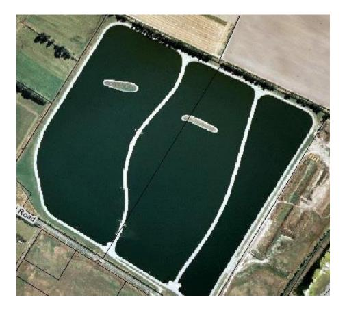
Our primary pond system is actually made up of 2 primary ponds running in parallel before combining at the outlet to run through the secondary pond. The infeed to these primary ponds is usually set at a 50/50 split but at the time of this discharge 75% was being diverted to the first pond and only 25% to the second one. This was just pure luck for us as the second primary pond was only partially effected.
