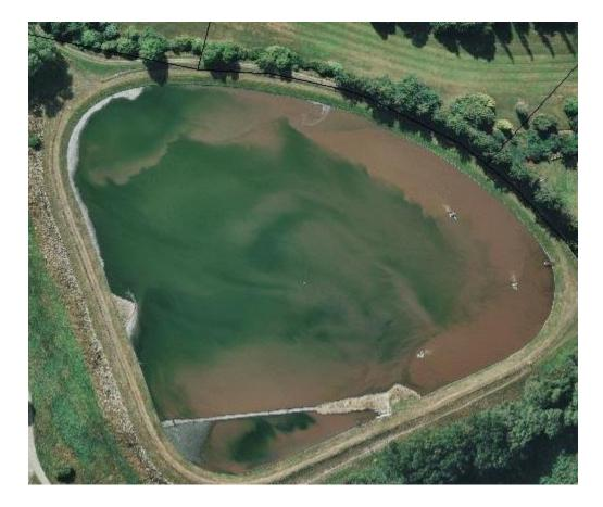
Within 4 months of this industry commencing discharge into this pond it was completely devoid of any algae and had been taken over by purple anaerobic bacteria which are sulphate bacteria that thrive in anaerobic conditions. These bacteria turned the whole pond pink and in the aerial photo (left) you can see it just as the pond is turning.
