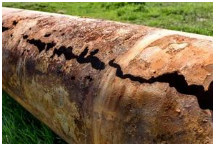
Figure 5. Corrosion of sewer pipes from acidity
