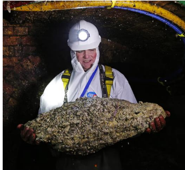
Figure 11. Fatberg found in sewer network.
